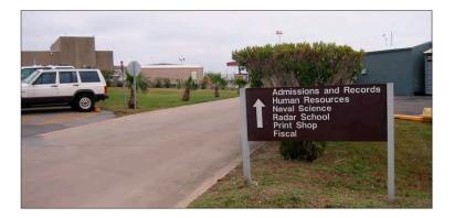
Campus signage oriented to motorists suffers from three major problems: (1) there are too many destinations listed; (2) the size of text is not sufficient to accommodate visibility at a reasonable distance, and (3) the signs themselves are not of a sufficient scale to accommodate the information they must carry.
