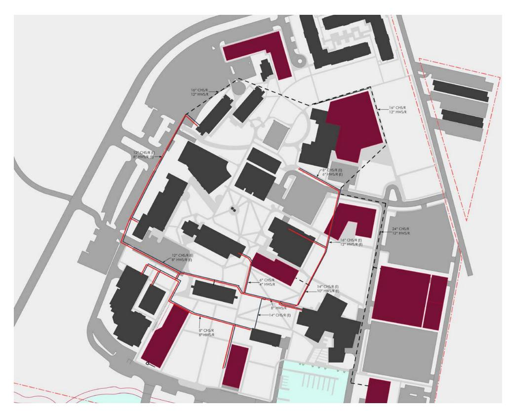
The campus currently has only 300 tons of firm capacity available. A new central plant or major expansion of the existing plant will be necessary to add any significant additional load to the campus loop. The build-out of the master plan requires a minimum of 3,200 tons for cooling and 14,000 MBH for heating, meaning that significant additional capacity will be needed.
